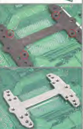
Place the "H" metal back plate directly over the "H" insulator.
